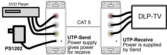
The UTP-Send uses very little power and is normally left on. A led lamp shows if power is connected properly to the UTP-Send.
