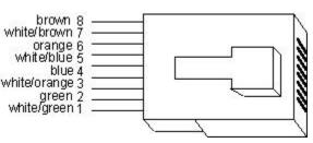
are connected using a single cat 5 wire using all 8 conductors. Connection is made with the RJ45 connector (RJ45 plug not supplied). Always use standard cat 5 wiring practices. Using the correct wire pairs and polarity is **VERY** important.
